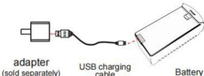
Please try to use an adapter with a charging current of 2A for charging, which can improve the charging speed.
